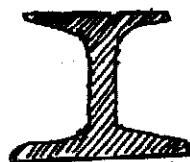
Fig. 8.17: Shape of cross-section of girder
