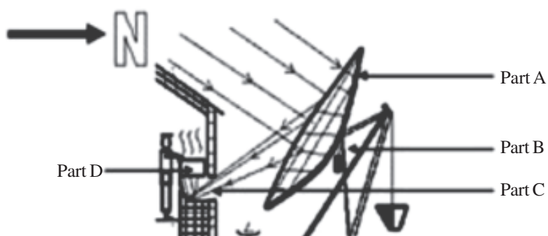
Fig. 31.6: Scheffler community cooker concentrator
