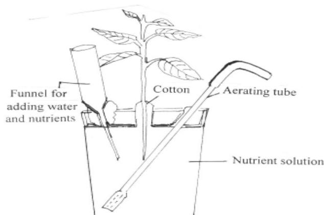
Fig. 9.1 Experimental set up for nutrient solution culture of plants.
